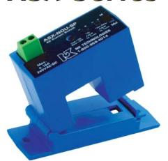
The 'ASX' Series from NK Technologies is a high-performance current-operated switch with field-adjustable time delay to help minimize nuisance trips during start-up and operation. Designed for motor status applications where setpoint accuracy and repeatability are critical, the ASX offers a linear setpoint characteristic and constant hysteresis. Standard features include self-powering, jumper-selectable ranges and a choice of outputs and cases.
