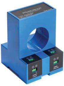
DT Series, Large Aperature Current Transducers combine a Hall effect sensor and signal conditioner into a single package for use in DC current applications up to 1200A. The DT Series has factory set and calibrated ranges and industry standard 4–20mA, 0–5VDC or 0–10VDC outputs. Available in solid-core DIN rail mounted enclosure.
