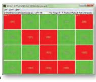
It does not matter how many features are inspected. If any feature on a part is out of specification, that part is considered a bad part. QC-Sort displays the corresponding rectangle for that part in red. All good parts are displayed in green.
